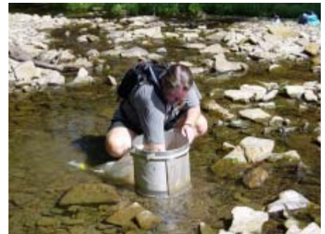
Using a Hess Sampler, Robin Reese collects macroinvertebrates at Winn Creek, a tributary of the West Fork White
